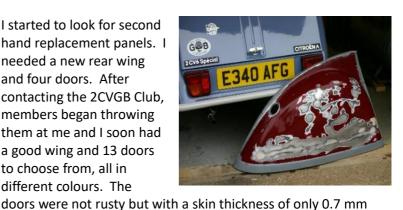
they all had many small dents. They sometimes split along the top edge and getting rid of dents is like working on a large biscuit tin lid. The front doors are on hinges but the rear ones are held on by gravity and can be slid off vertically. I was able to keep the bonnet and that too has no hinges and can be slid off sideways. The existing boot lid was good.
